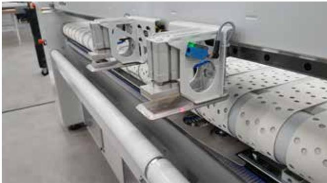
Each spreader clamp is controlled by a servo motor for maximum productivity and accuracy. Also the horizontal movement is servo-controlled.
