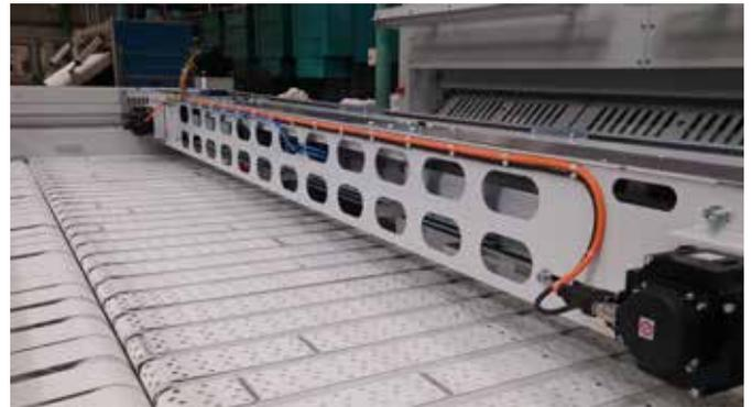
Beside the vacuum box, there are also a high spinning in-feed roller, stretch knife and spreader brushes, all contributing to a smooth shake out and spreading performance.
